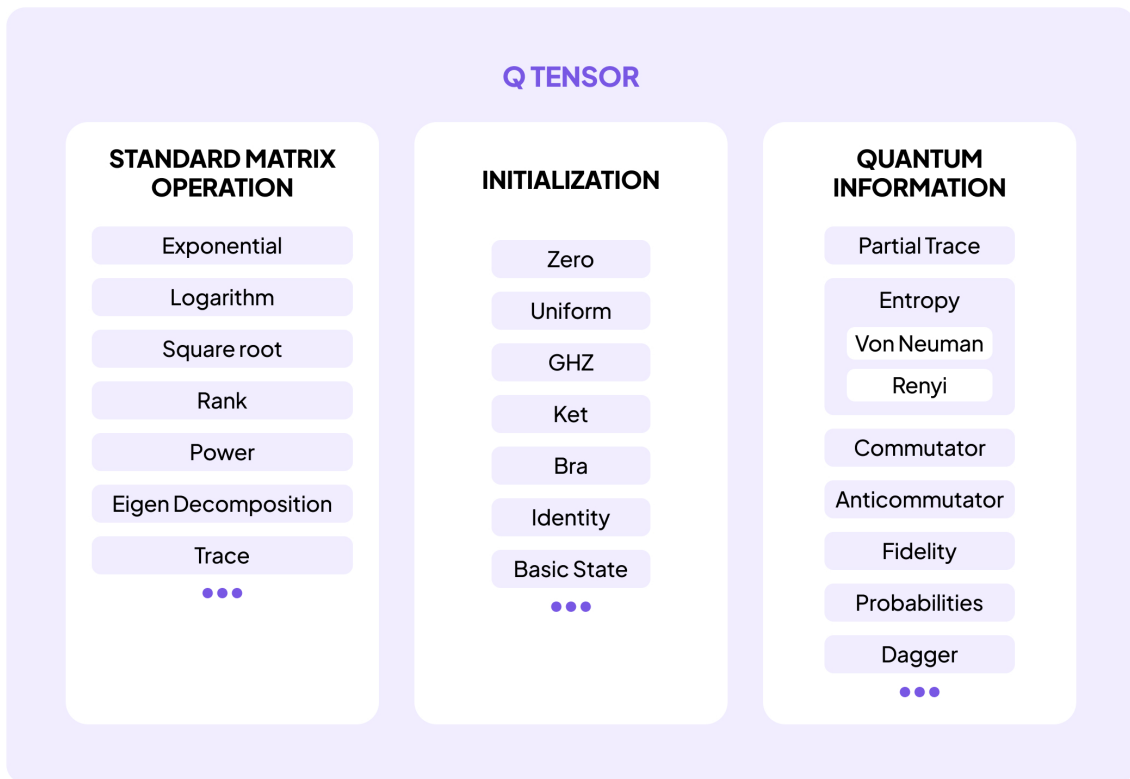
Figure 5.1: An overview of the QTensor class operations. QTensor is QiliSDK’s core data structure for representing quantum states and operators in sparse form, supporting kets, bras, density matrices, and scalars. Its operations are grouped into standard matrix operations (exponential, logarithm, square root, eigen decomposition, trace, and more), state initialization helpers (zero, uniform, GHZ, ket, bra, identity, basis state), and quantum-specific operations (partial trace, entropy, commutator, anticommutator, fidelity, and probabilities).
